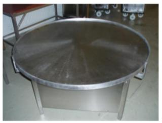
The Havantec turntable is ruggedly constructed of stainless steel. The table is equipped with one speed and therefore has one speed of 3.1 RPM (rotations per minute) Optionally it can be supplied with a heavier motor or frequency controlled.
